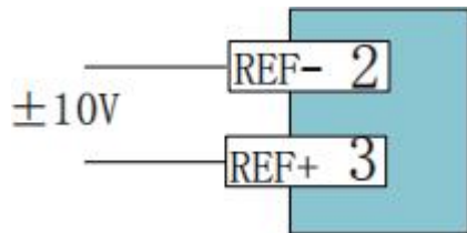
Figure 4.3.2 Analog input wiring of external power supply
