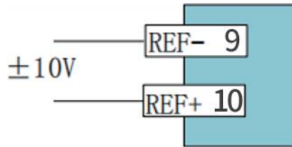
Figure 4.3.2 Analog input wiring of external power supply
